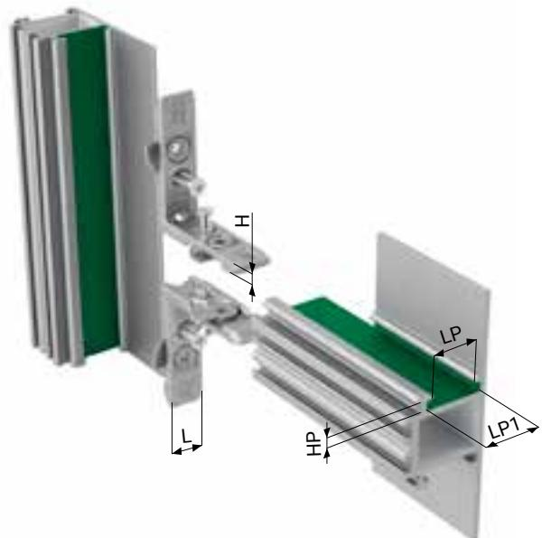
Internal alignment corner joint for quick assembly on Euro groove, in die-cast aluminum with adjustable cams and tightening screws. Designed for T and cross junctions, it can be installed on assembled profiles without any processing. It has specific glue channels to guarantee perfect sealing and greater strength while avoiding any waste or spill.
